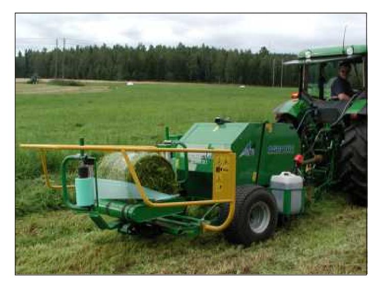
The AGRONIC 60/70 COMBI is constructed the same way as the mini-baler, but it is equipped with an automatic wrapper that efficiently wraps the material immediately after the material is baled.
