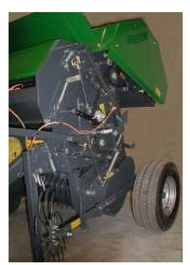
The baler is a fixed chamber baler with a net applicator. The density of the bales is adjustable by a mechanical chamber lock.
